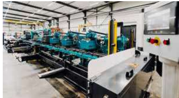
The All-in-One machines produce the screws continuously, directly from the coil.
