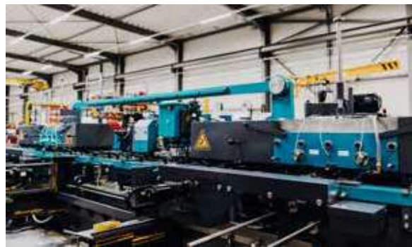
The new-generation machines produce eighty 420-mm-long, 10-mm-diameter (OD) full-thread screws per minute.
